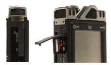
**HOW TO REMOVE THE CARD:** Gently press the SD card inward, and then release your finger. When the SD card pops out, remove it.
